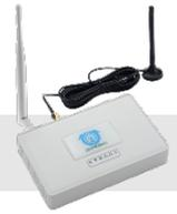
1 Remove yellow cap and screw on **black mobile radio antenna**
