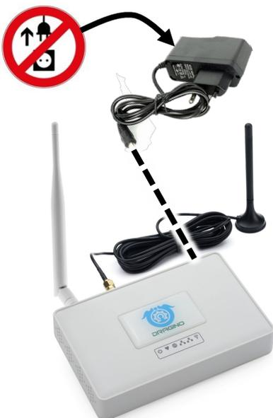
3 After plugging in, the gateway **boots up** and establishes a LoRa network
