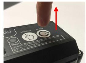
After switching on, the device connects to the WiFi network and sends a first image. This process usually takes no longer than **1 minute**. Your TOM device then appears as online in the traplinked app.
